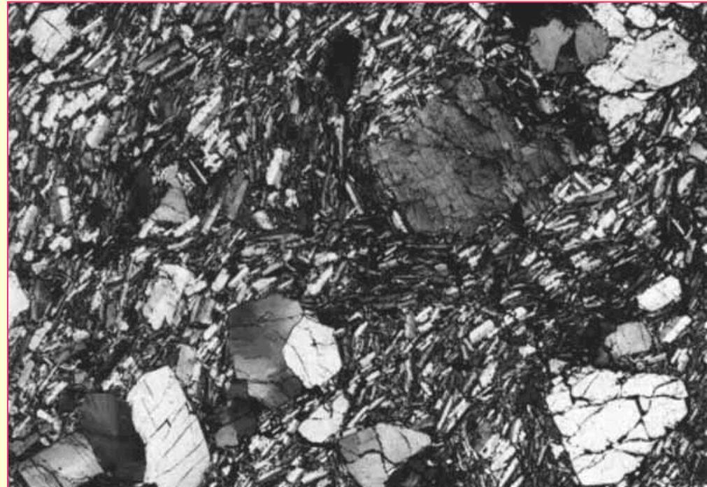
Figure 3.12a. Trachytic texture in which microphenocrysts of plagioclase are aligned due to flow. Note flow around phenocryst (P). Trachyte, Germany. Width 1 mm. From MacKenzie et al. (1982). © John Winter and Prentice Hall.
