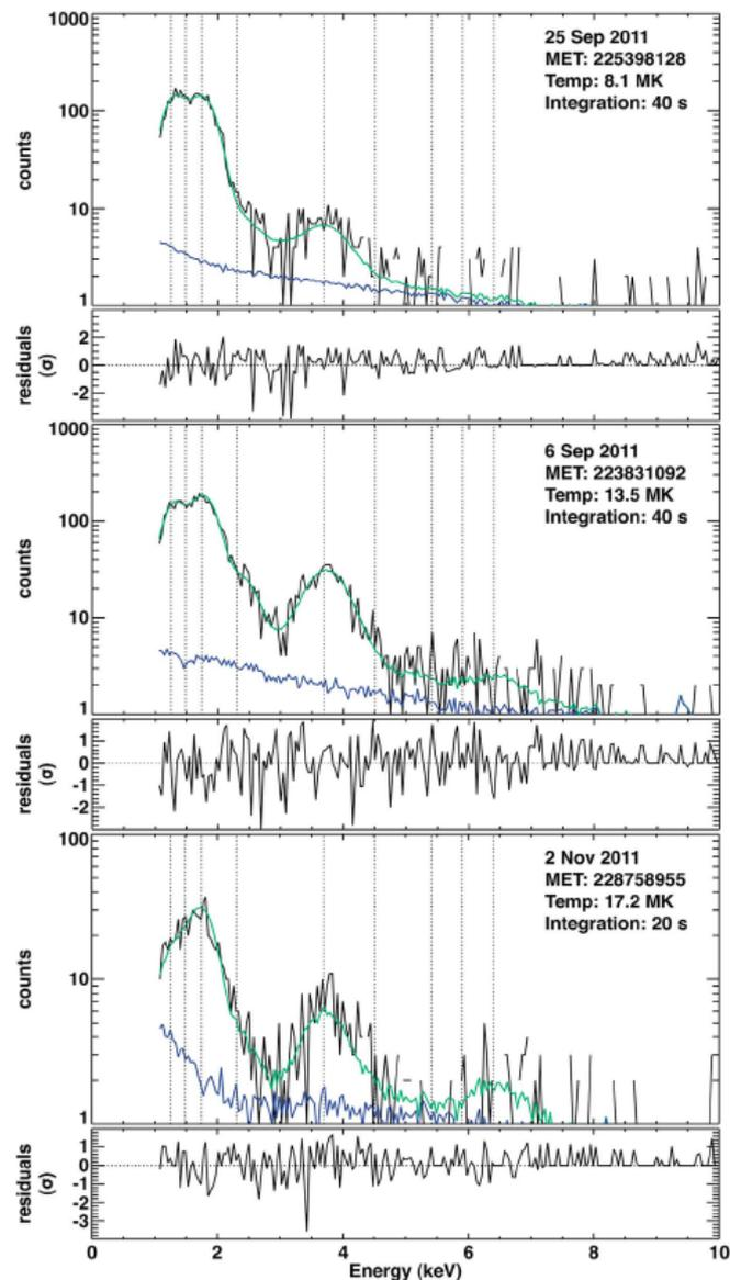
**Figure 1.** Three examples of fits to solar flare X-ray spectra measured by the SAX. The steeply inclined green line depicts the electronic background in the detector; the red line is the best fit solar spectrum (for the plasma temperature given in each case) convolved with the instrument response. The Ca and Fe line complexes (at  $\sim 3.6$  keV and  $\sim 6.4$  keV, respectively) increase in magnitude with temperature. MET = mission elapsed time, in s.
