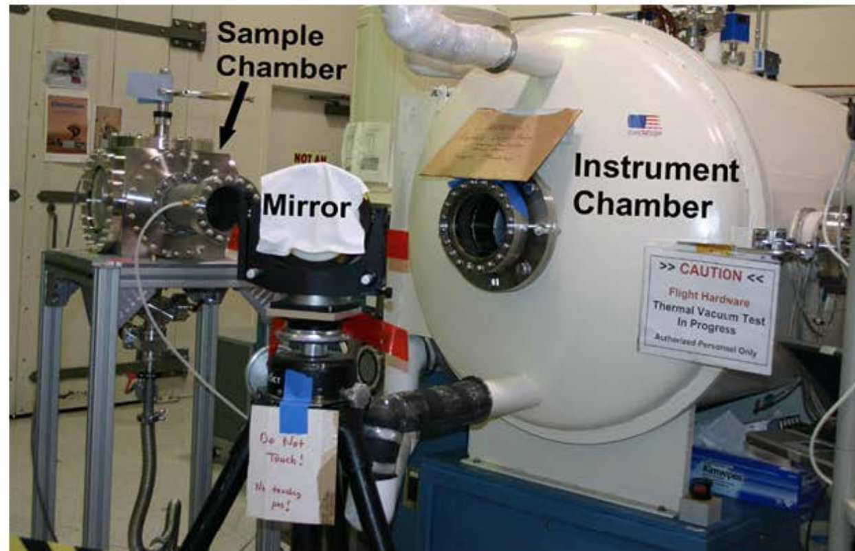
Fig. 23 Experimental set-up for ChemCam LIBS thermal vacuum tests. The instrument is in the large white thermal chamber to the right, a turning mirror is in the foreground, and the sample chamber is to the left, providing an instrument-to-sample distance of 1.5 m. For tests with more distant sample positions the sample chamber was moved back, into the adjoining room
